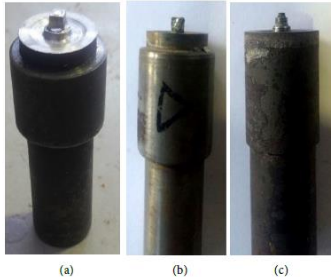
Figure 2. FSW tools shapes. (a) Square;(b) Triangular; (c) Stepped.[8]
