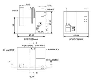
Fig-1: Plan and section of model (all dimensions are in cm)
