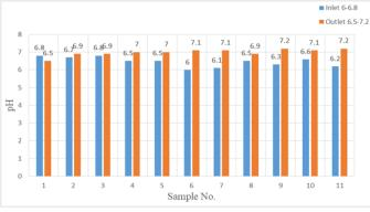
**Chart-1:** pH results from inlet and outlet samples
