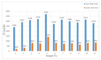
**Chart-5:** TS results from inlet and outlet samples
