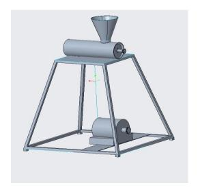
The manufacturing process used in fabrication of the oil extracting machine from nuts is such that the total cost of fabrication is reduced and also one that can make use of the available materials. The manufacturing process involved in this work includes, joining of metal parts by welding, cutting
