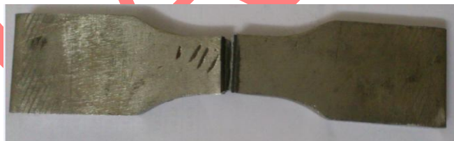
Fig 4: Tensile test specimen after test
