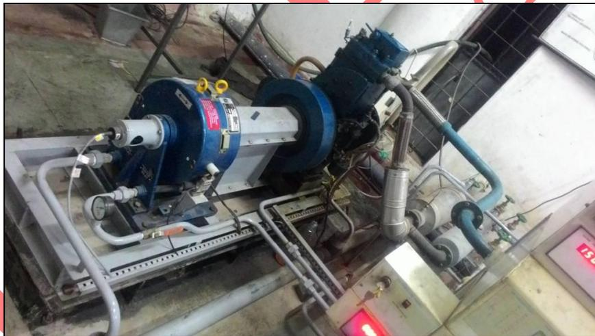
Figure 2 Pictorial View of EGR Setup
