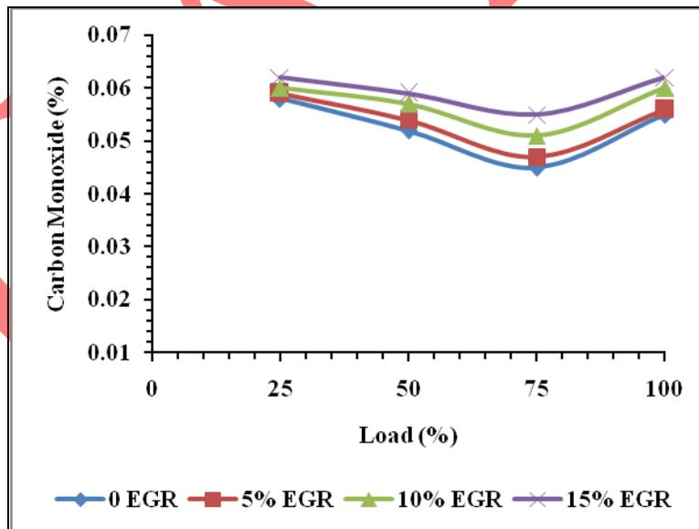
Figure 5 Variation of CO with Engine Load
