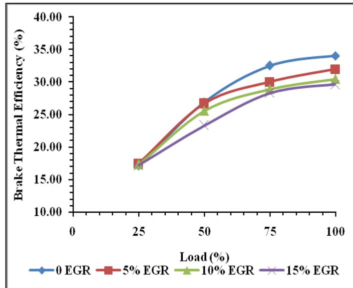
Figure 4 Variation of BThE with Engine Load
