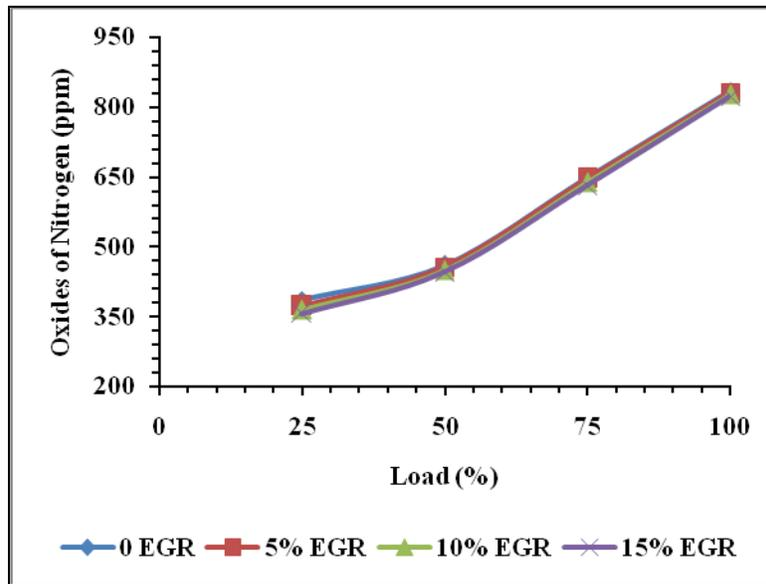
Figure 7 Variation of NO<sub>x</sub> with Engine Load
