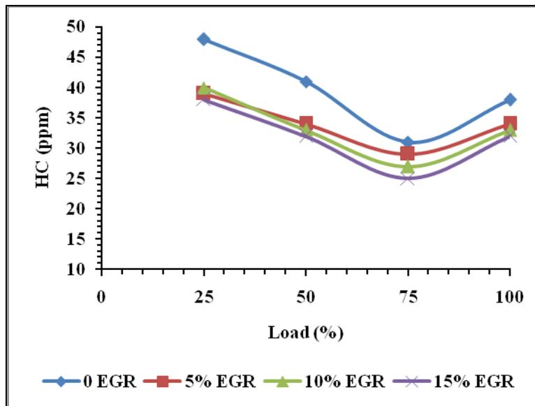
Figure 6 Variation of HC with Engine Load
