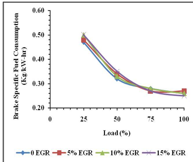
Figure 3 Variation of BSFC with Engine Load
