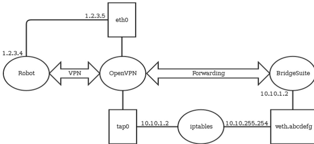
Fig. 2. Robot connection.
