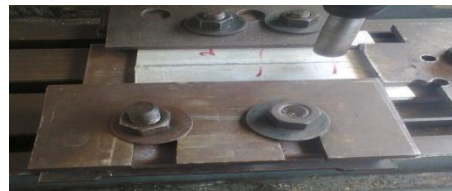
Fig.4 Setting the Al plates in Universal Milling Machine
