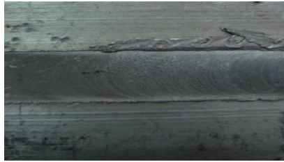
Fig.5. Al plates join by FSW
