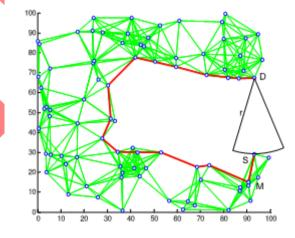
Fig 3.1 In GR, node S cannot find any other node that is geographically closer to the destination D.
