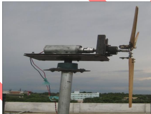
Figure.5 Assembling of DC Generator and Hub
