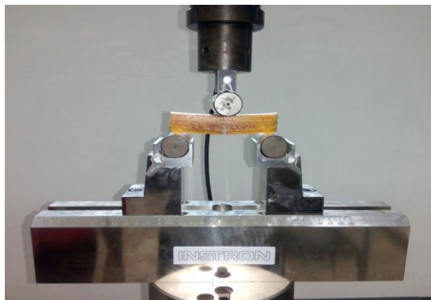
Figure 3. Testing of sample on INSTRON UTM using a 3 point bending fixture.
