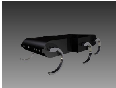
Fig. 1. Basic design outlook of the bot in standing position using its C-Legs.
