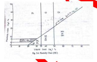
From the liquid limit test, the soil is greater than 50%. So the soil having the high compressibility. From the A-line chart we classified that the soil is CH (inorganic clay of high plasticity).
