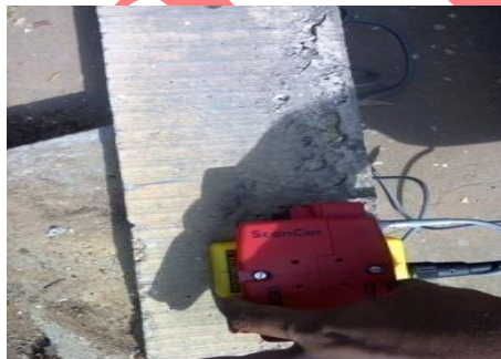
Fig 5.2. Testing of Cover Thickness using Scanlog.
